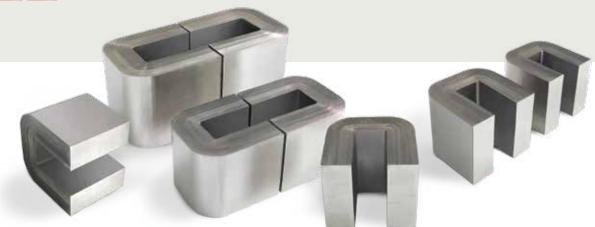
Amorphous cut cores are made from metallic glass materials without a crystalline structure (as seen in silicon steels, permalloys, orthonol, and nanocrystalline cores). The amorphous atomic structure results in much higher resistivity than what is exhibited by crystalline alloys; therefore, amorphous cut cores offer excellent frequency response and efficiency.
