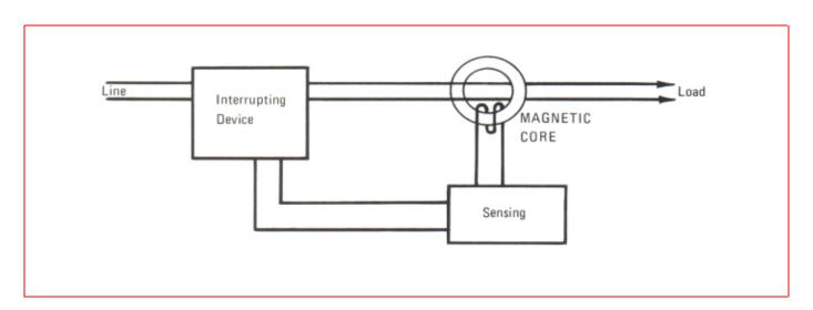
The heart of a ground fault detector is a high initial permeability magnetic core with a sensitivity capable or detecting minute differences in currents entering and leaving a load. The following are typical core requirements for meeting GFI specifications:
